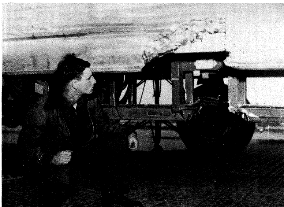
Eighteen inches of catwalk chewed out by a propeller
