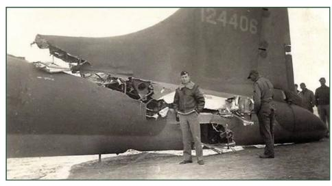
control cables were severed, except one single elevator cable still worked, and the aircraft still flew...miraculously! The tail gunner was trapped because there was no floor connecting the tail to the rest of the plane. The waist and tail gunners used parts of the German fighter and their own parachute harnesses in an attempt to keep the tail from ripping off and the two sides of the fuselage from splitting apart.
